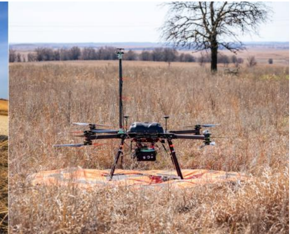
Fixed-wing UAV equipped with magnetometer and Rotary UAV equipped with wind speed and methane sensor
