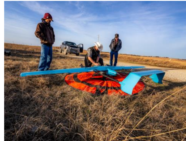
Fixed-wing UAV equipped with magnetometer and Rotary UAV equipped with wind speed and methane sensor
