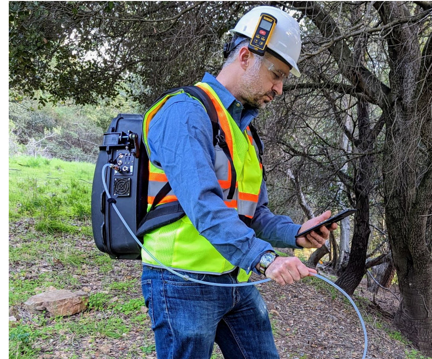
Backpack Gas analyzer used to locate methane point sources (credit: Sebastien Biraud, LBNL)
